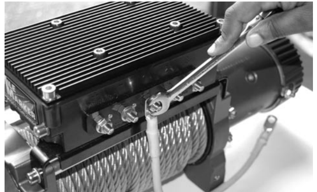
2-8: Attach Cable and Tighten with 13 MM Wrench. Repeat per schematic.
