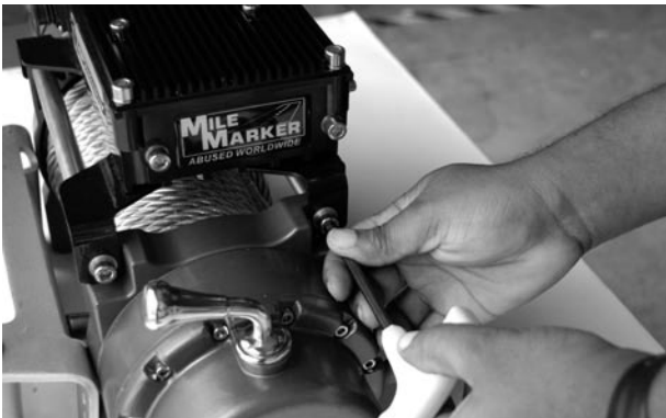
2-6: Once all points are mounted, TIGHTEN ALL FOUR BOLTS.
