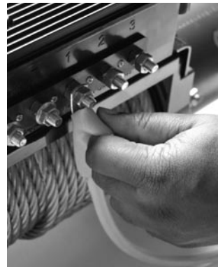
2-9: Affix boot over cable connection. Be sure boot completely covers electrical connection. Repeat for all connections.
