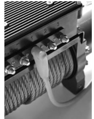
2-9: Affix boot over cable connection. Be sure boot completely covers electrical connection. Repeat for all connections.
